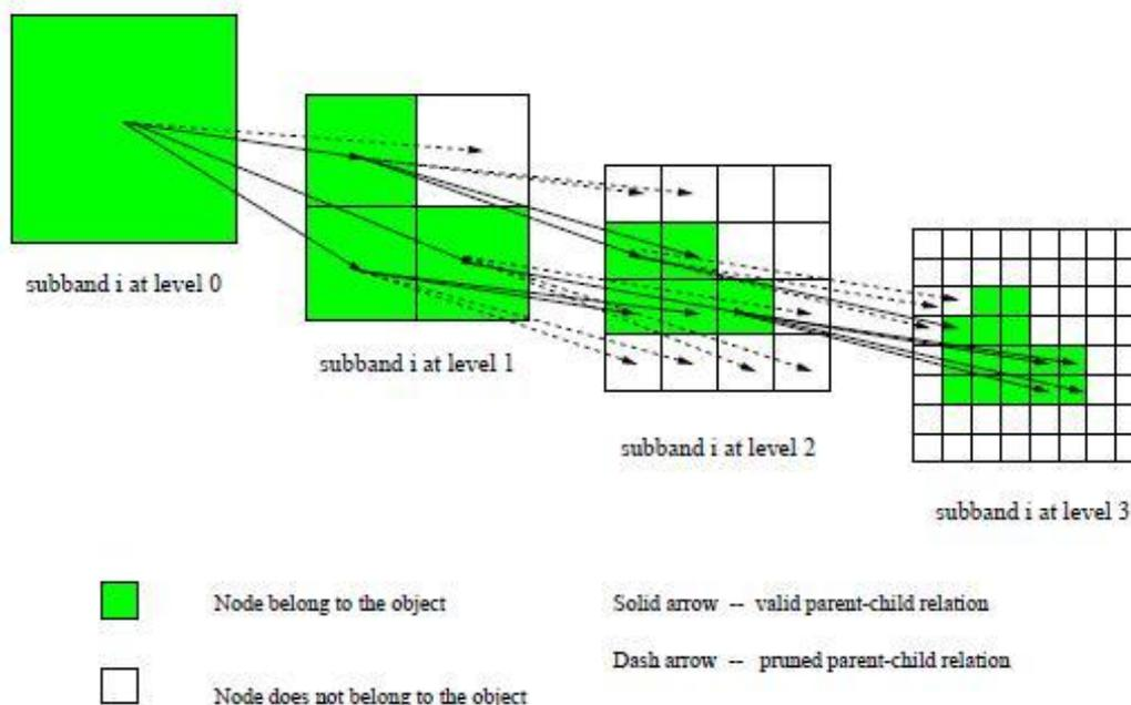
In the parent-child relation in the OB-SPECK algorithm, the branches, which correspond to the nodes outside the object (represented by the dash arrows), are pruned before the coding process begins.
